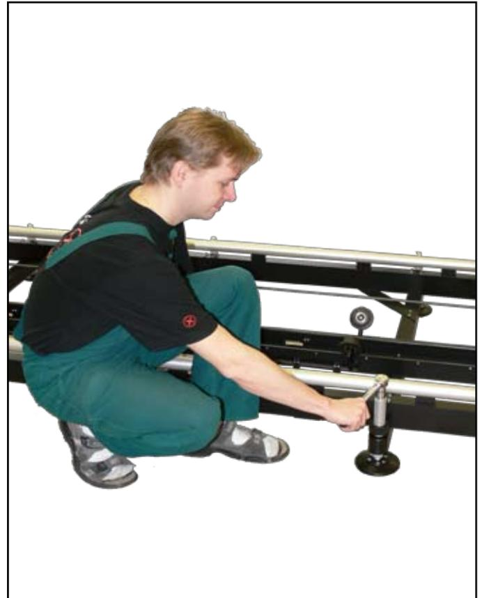
2.2.2.c. Leveling jacks fitted along the track
