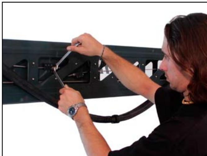
2.6.1.f – Securing nut with two spanners
