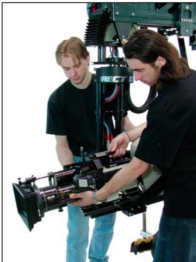
2.9.2.a - Mounting camera on the base plate
