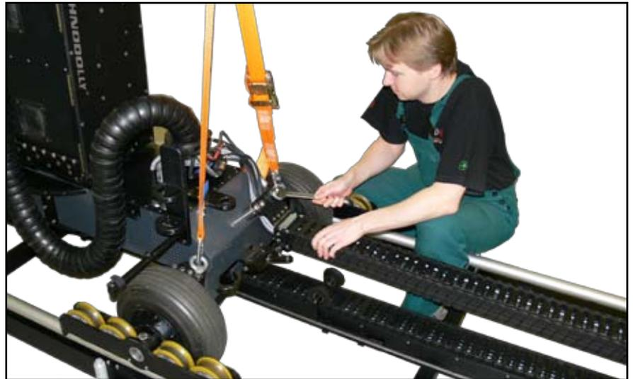
2.2.6.e. - Attaching the cable carrier to the base
