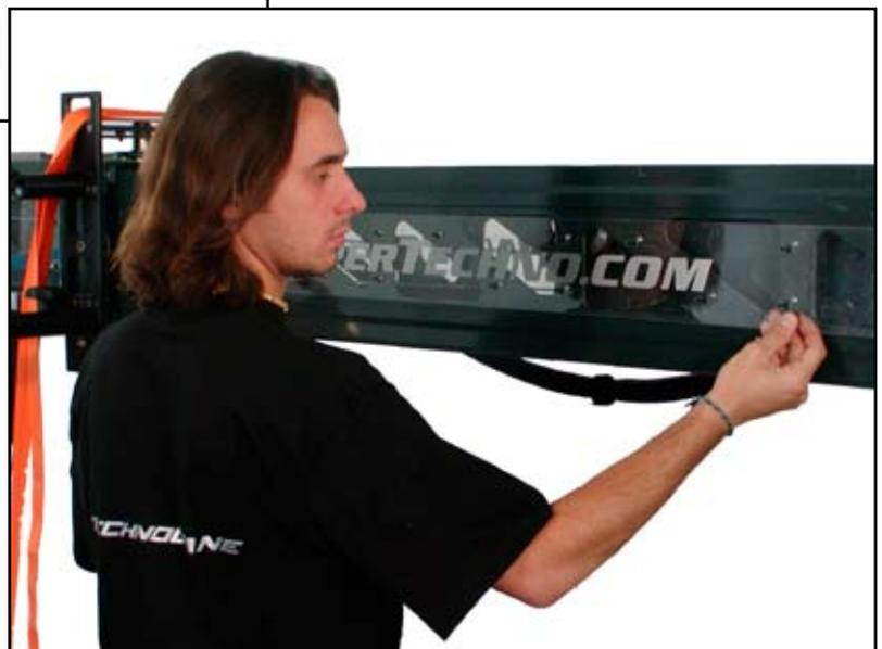
2.4.1.b – Removing the plastic shield
