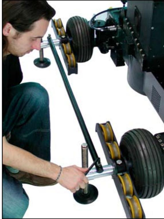
1.2. - Locking steering with the locking bar
