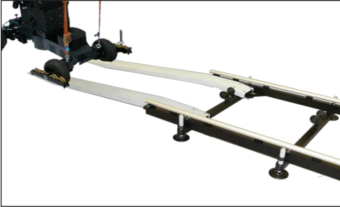
*2.2.4.b – Base moving onto the ramps*
